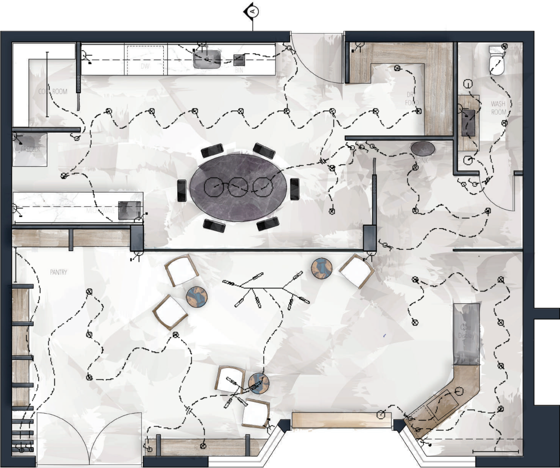
FLOOR PLAN ELECTRICAL LIGHTING PLAN 1:50
