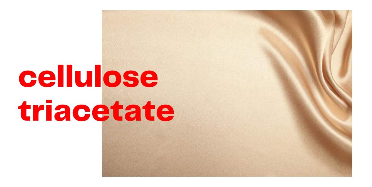
low-cost fibre produced from cellulose (wood pulp or cotton linters) which then chemically processed with acetic acid
