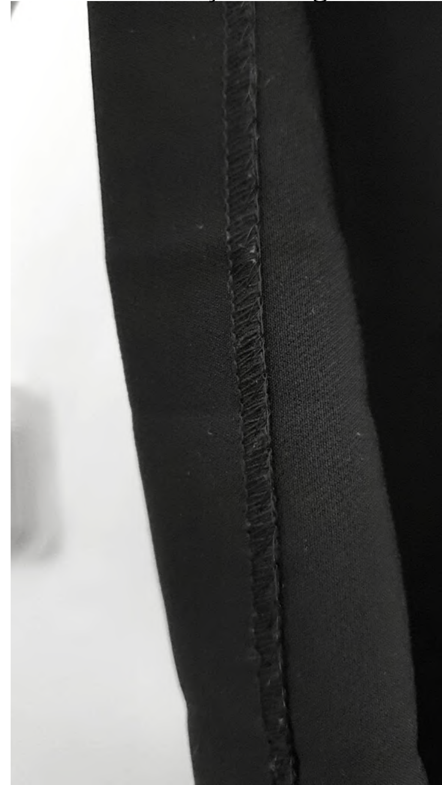
Overlock and blind catch stitch finishing
